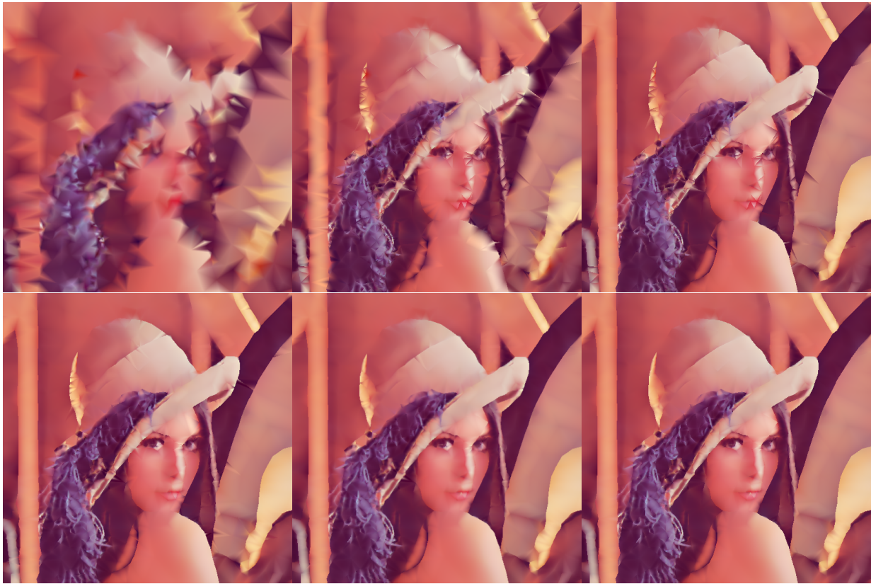
Figure 5.8: Progressive image reconstruction state after partial decoding of the bitstream. Here follow the decoded bitstream percentage from left to right and top to bottom: 35%, 67%, 76%, 90%, 96% and 100%.
